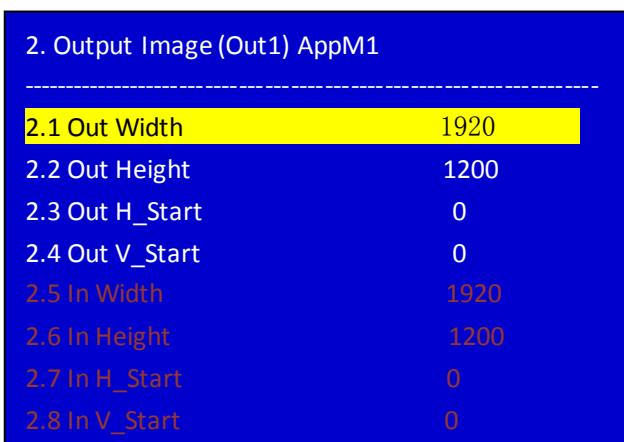
13.3. In the setup menu **In width and height**, **In H-start and V-Start** used to crop the area of input video source then output the area, normally we don't use it;
