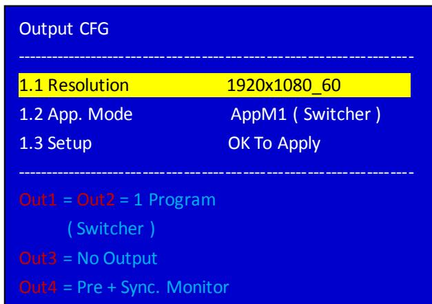
11.3. normally the output resolution must be bigger than the actual resolution of LED screen or equal, for example the LED screen ( resolution 1792 X 1056) which connects to Out 1, so the output resolution we set must be bigger than this one, 1920 x 1080 resolution will be ok for this;
