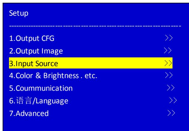
16.2. Press **Brt+** or **Brt-** button to select setup option, rotate **OK** to select input source, press **OK** to save;
