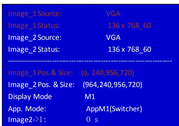
17.2. Press **Setup** button to enter PIP parameter configuration menu, press **Brt+** or **Brt-** to select setup option **D.1 Image\_1 source** or **D.2 Image\_2 source**, rotate **OK** to configure input video source, press **OK** to save;
