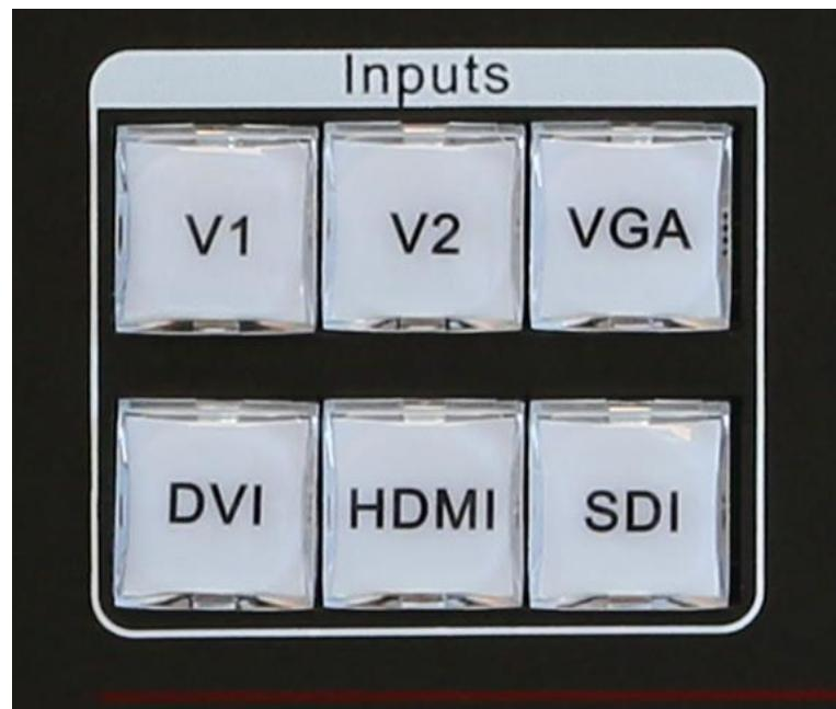
1.1. LVP909 has 6 channels of input port: **V1 V2 VGA DVI HDMI SDI**;
