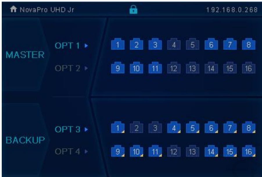
Figure 4-3 Optical fiber port statuses – Hot backup
