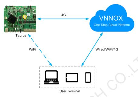
VNNOX could be accessed directly or by way of bridge connection to centrally manage post screens.
