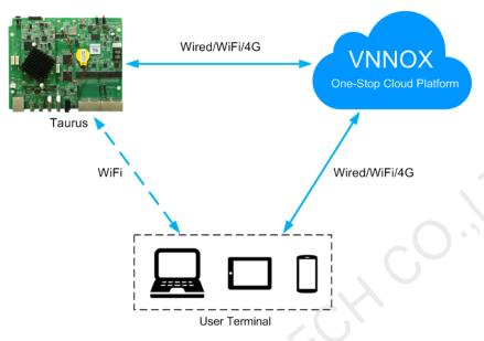
VNNOX could be accessed directly or by way of bridge connection. When bridge connection is selected, following three methods for Internet connection of Taurus products are available with priorities ranging from high to low:
