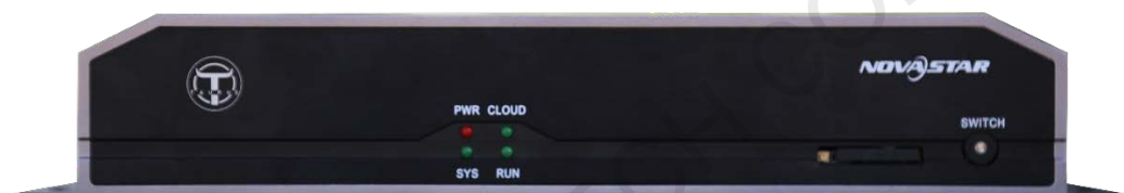
Figure 3-1 Front panel of the TB6
