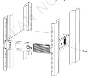
Elevated Operating Ambient - If installed in a closed or multi-unit rack assembly, the operating ambient temperature of the rack environment may be greater than room ambient. Therefore, consideration should be given to installing the equipment in an environment compatible with the maximum ambient temperature (Tma) specified by the manufacturer.
