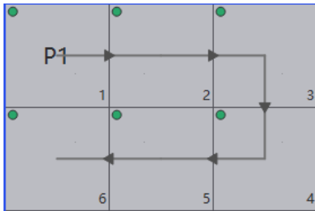
Figure 5-3 Cabinets connected automatically
