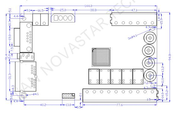
Tolerance: ±0.1 Unit: mm
