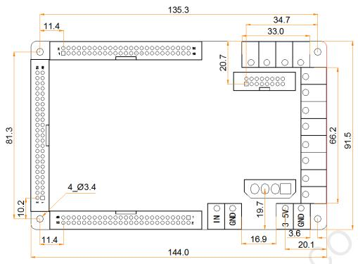
Tolerance: ±0.1 Unit: mm
