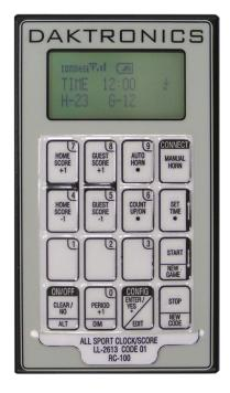
The RC-100 handheld controller is a truly wireless device that can control a variety of Daktronics standard scoreboards. For baseball/softball, the umpire operating the RC-100 unit, as well as the fans and players, can instantaneously see the ball and strike count on the scoreboard. For tennis, multiple RC-100 units can be used to control multi-court scoreboards.
