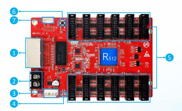
$\Phi$ : Gigabit Ethernet port, used to connect the sending card or receiving card, the same two network ports are interchangeable,
