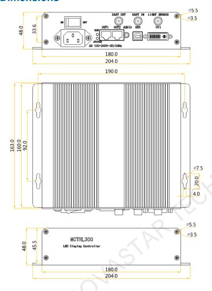
Tolerance: ±0.3 Unit: mm
