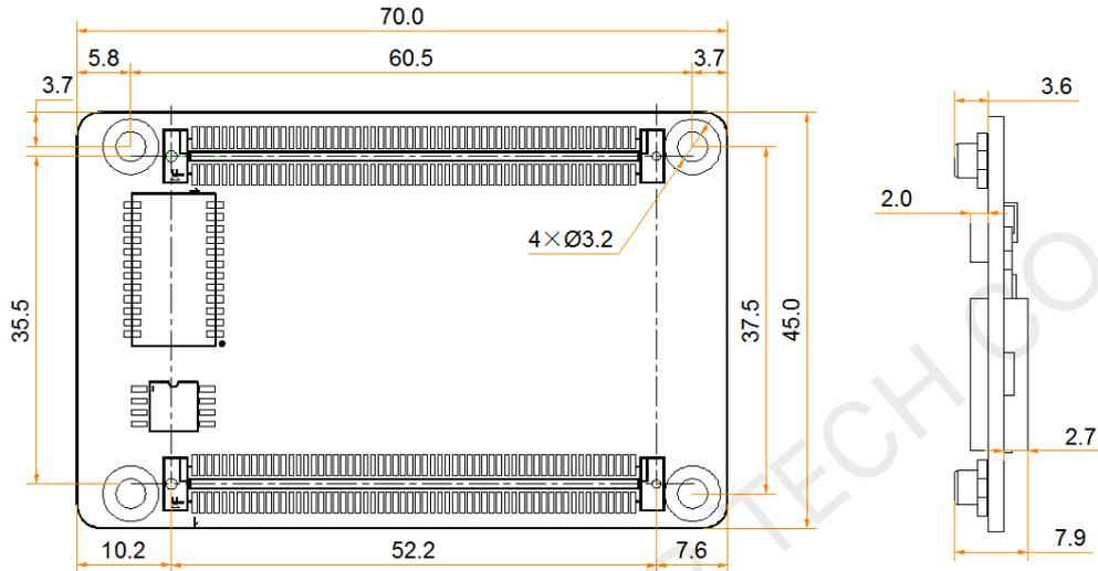
Tolerance:  $\pm 0.1$  Unit: mm
