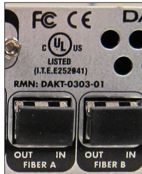
Figure 4: Rack-Mount Fiber-Optic Ports
