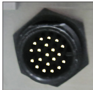
Figure 9: Display-Mount Power Input
