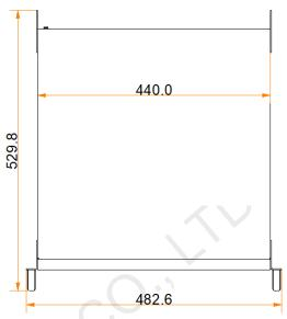
Tolerance: ±0.3 Unit: mm
