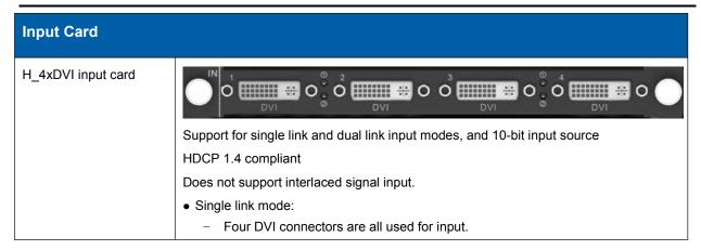
Each connector supports the maximum resolution of 2048×1152@60Hz and the minimum resolution of 800×600@60Hz.
