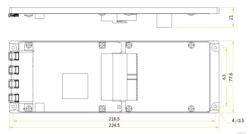
Tolerance: ±0.3 Unit: mm
