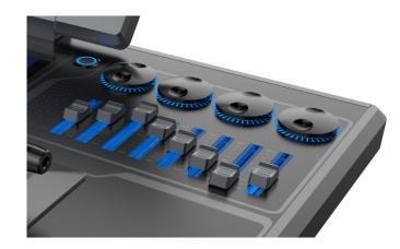
Four encoders and eight faders make the event operations unrivaled convenient. Also, the encoders and faders can be bound with external MIDI functions for volume adjustment and more.
