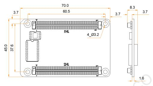
Tolerance: ±0.3 Unit: mm
