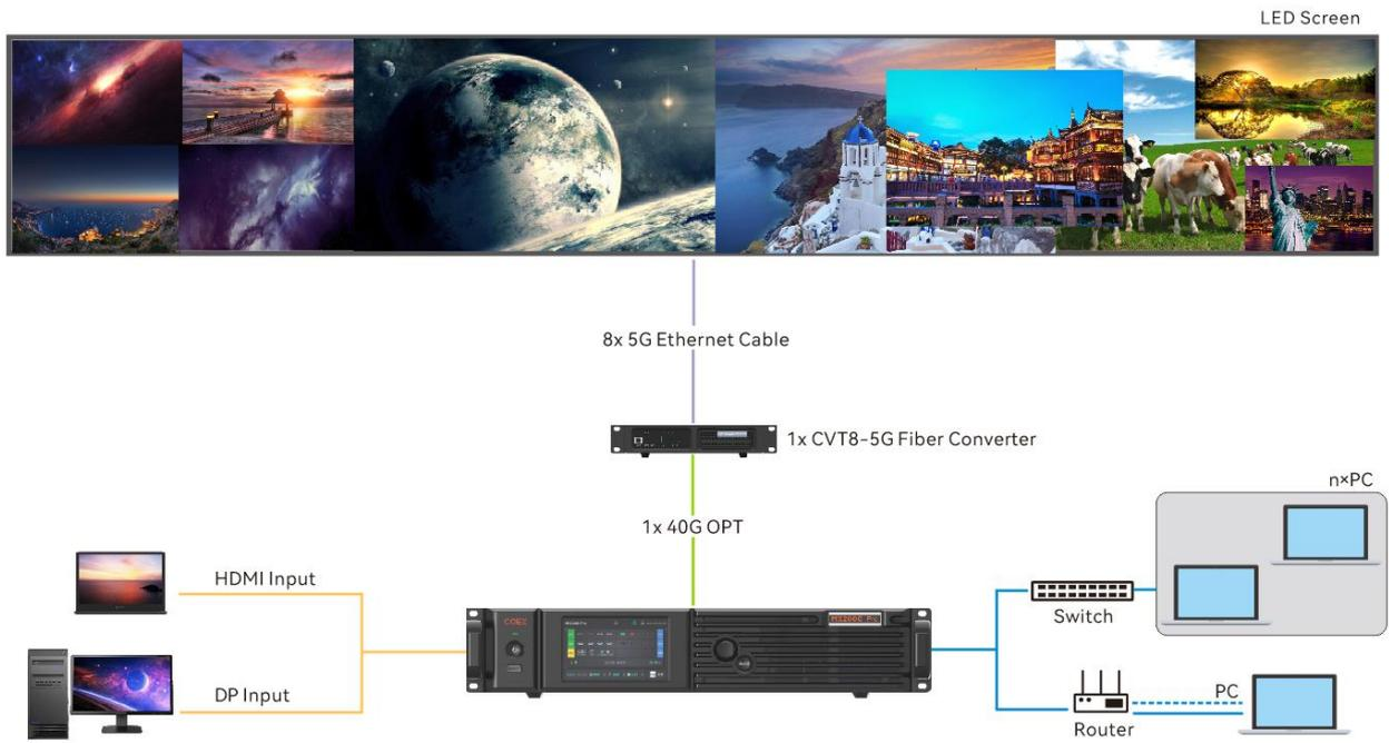
This diagram is an example of two input cards and one CX\_1x40G\_Fiber output card installed on an MX2000 Pro. The actual application may vary.
