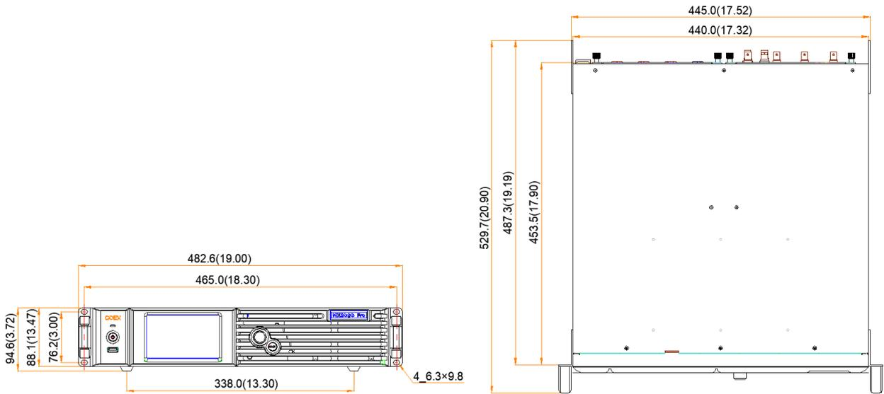
Tolerance: ±0.5 Unit: mm
