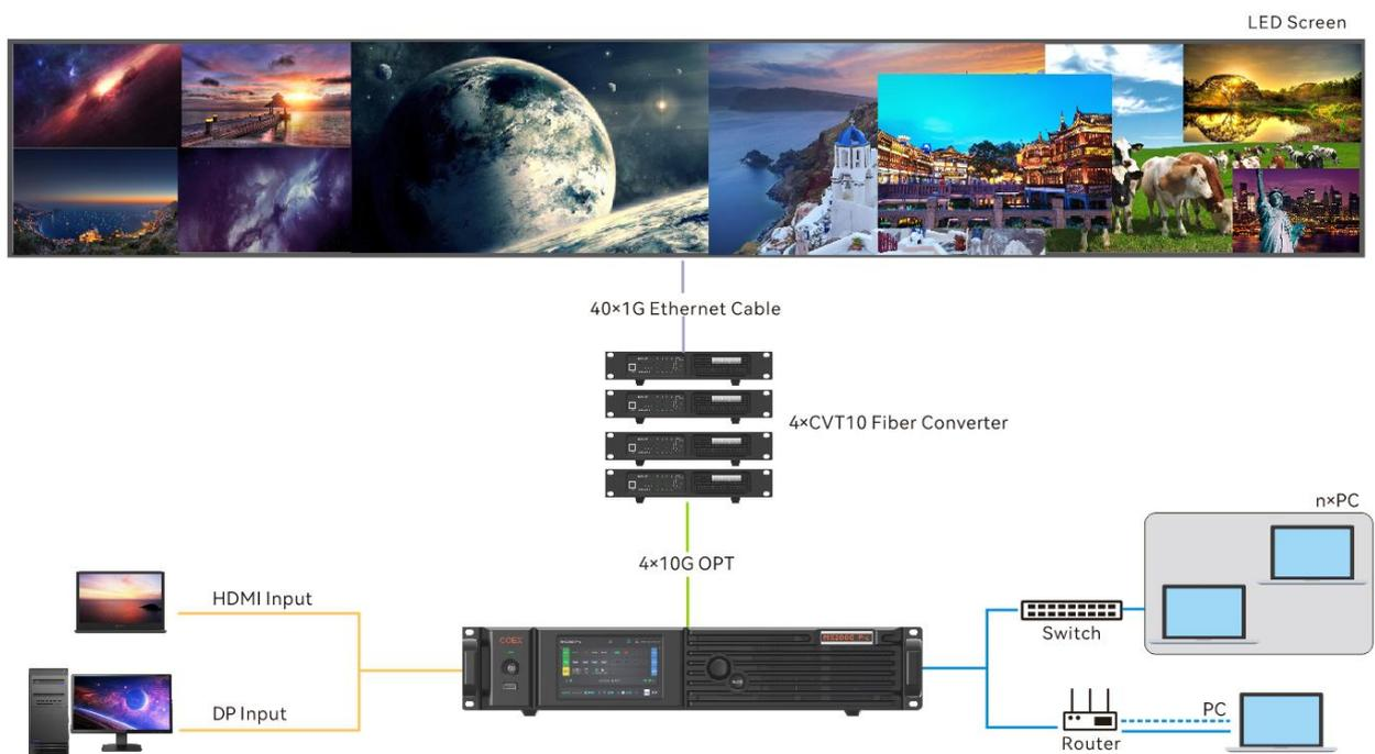
This diagram is an example of two input cards and one MX\_4x10G\_Fiber output card installed on an MX2000 Pro. The actual application may vary.
