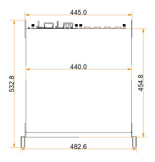
Tolerance: ±0.5 Unit: mm
