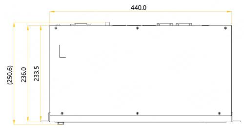
Tolerance: ±0.3 Unit: mm
